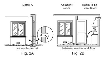
The air inflow may also be obtained from an adjoining room, (provided the latter is not a bedroom or a room where there is a risk of fire, such as garages, fuel stores, etc.) which is ventilated in compliance with the standards in force.
